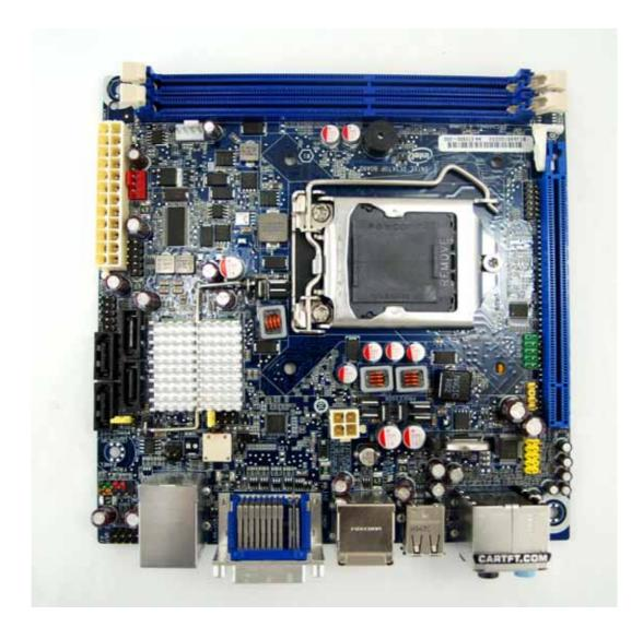
As mentioned in the specification you can find some more usefull connectors onboard. So you can find for example six USB (3 via Pinheader), four SATA (RAID functionality), one eSata and one PClexpress port.
