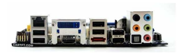
The backside of the new Mainboard looks very good. Additional to the standard I/O ports you can find a DVI, one HDMI, one eSATA and one SPDIF Connector which can realize a lot of different usages.
